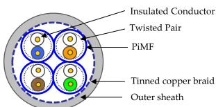
Fig 1. Cross Sectional Diagram of Cable
