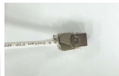
6. Wrap the tinned copper wire around the designated position for Grd. – Completion-
