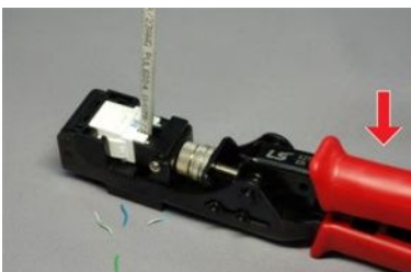
4. Squeeze the tool then Terminate all wires and trim the excess wires at the same time.
