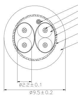
Ground wire: 11/0.18 tinned copper stranded Conductor: 7/0.24 tinned copper stranded Core wire: black. red; white. green (HDPE)
